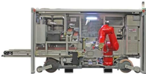
The SAM100 is a brick-laying robot, having already laid literally tons of bricks across the country on various industrial building and school projects. Under optimal conditions, SAM can lay up to 3,000 bricks per day, while a human can lay between 600 and 1,000. As just one example, while SAM was working on the Shenandoah University jobsite in Virginia, it set a world record for the most bricks laid in an eight-hour period, totaling 3,270!
